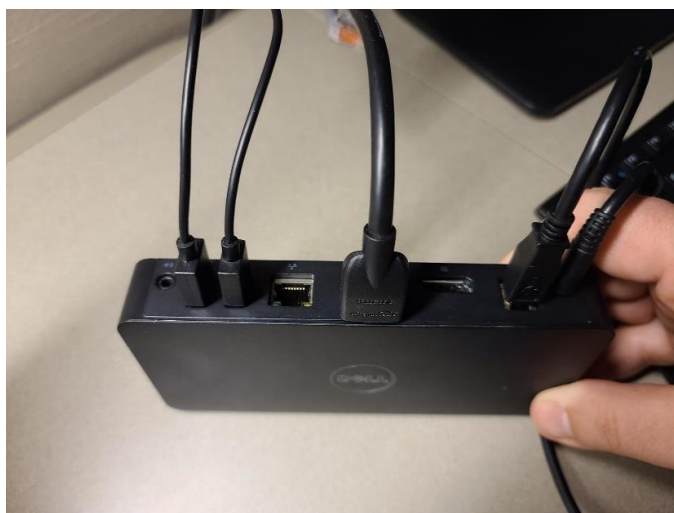
Image 2 - Behind the dock: from RIGHT to LEFT the power, USB from laptop, monitor, keyboard/mouse
